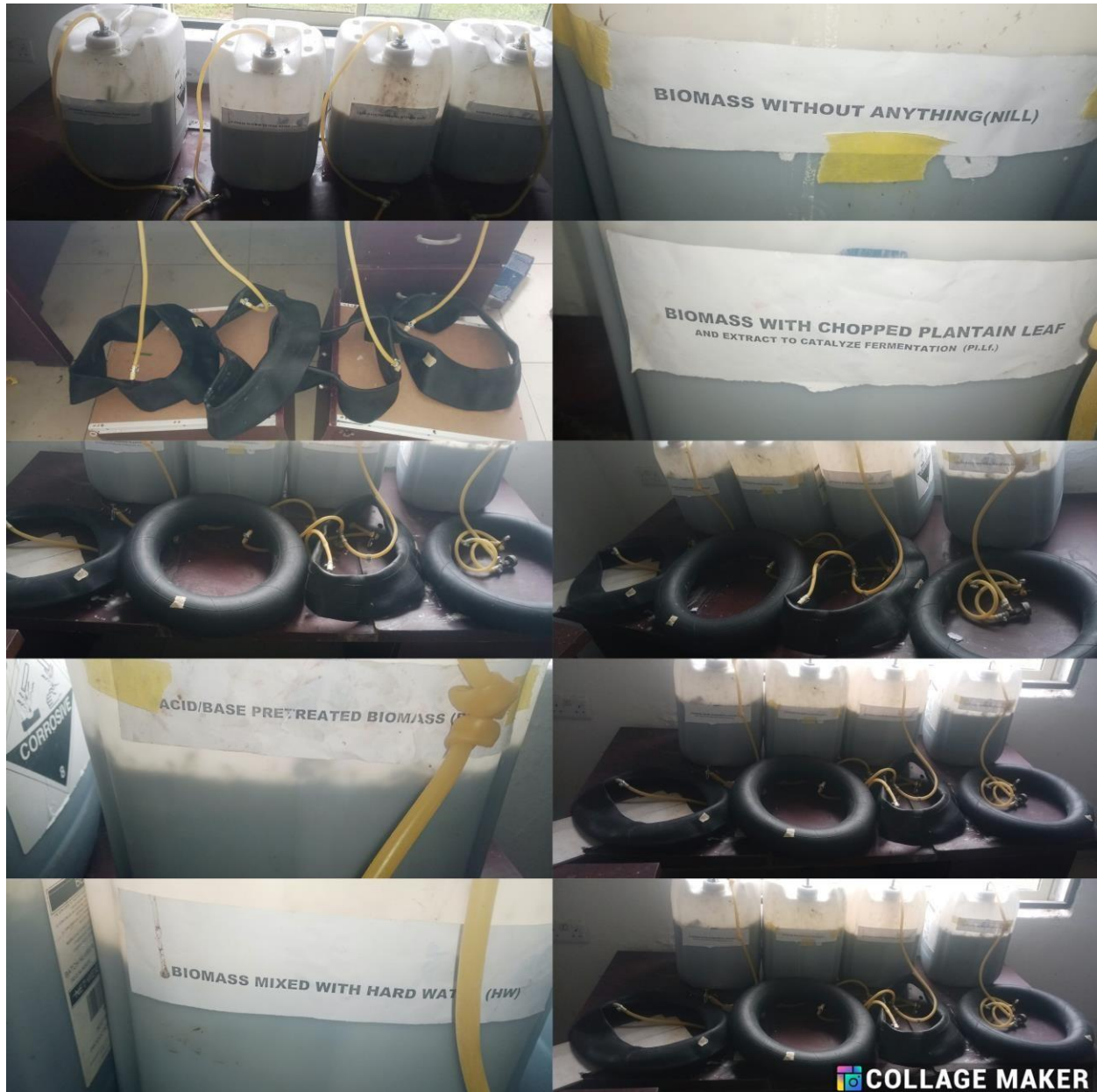
Figure 1 Locally fabricated digester with gas collection tubes fixed
